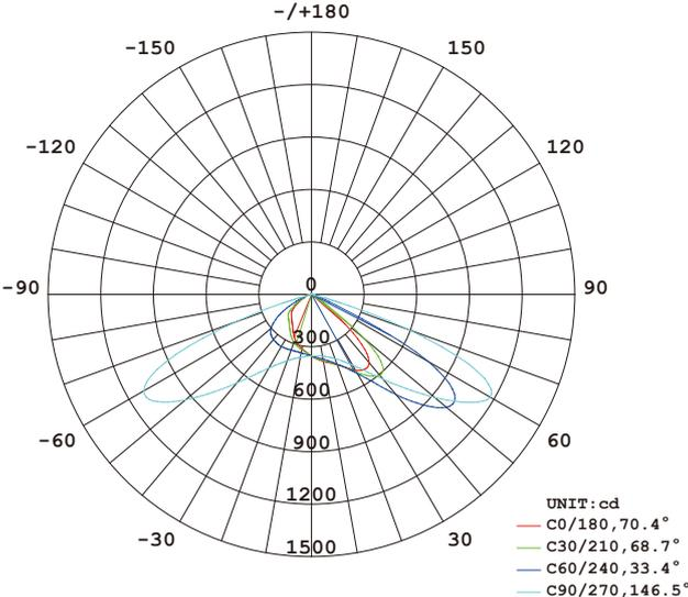
Beam Angle: X-axis: 158° Y-axis: 62°
